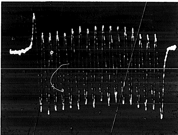
Fig. 6. Typical picture of the wiggler magnetic field measured using the pulsed-wire method.
